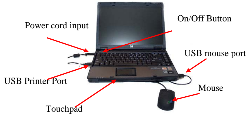
USB Port - printer to laptop connection
