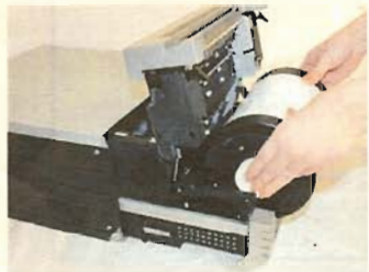
4. Set the paper holder into the printer's paper cassette. (Set it all the way in)
