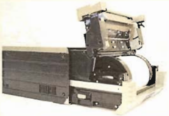
2. Open the Paper Release lever. Remove the scrap box
